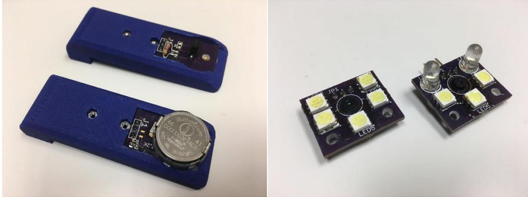
**Figure 45. (left) Sensor hoods populated with both the temperature and iButton sensors (left) and populated camera PCBs with both the patch and mixed LED lights for the lighting source of the mini inspection tool (right).**
