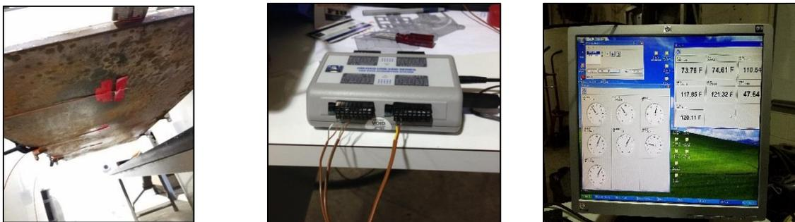
Figure 84. a) HSTs fixed under the plate b) DAQ system with thermocouples c) DAQ dashboard.
