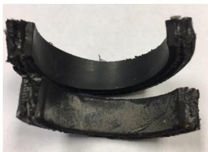
**Figure 106. Aged (bottom) vs. un-aged (top) coupons.**
