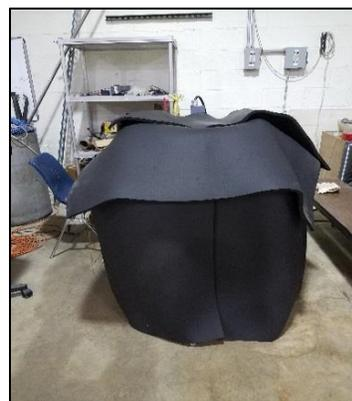
b) tank covered with insulation.
