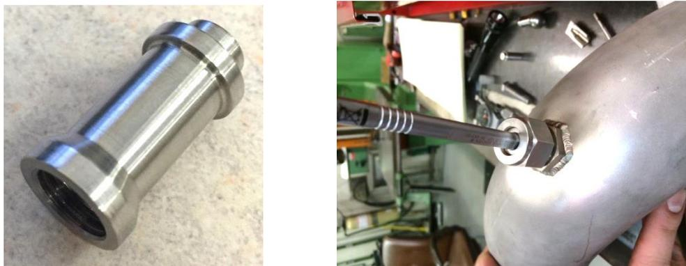
**Figure 95. a) Coupon, b) Coupon installed on an elbow.**
