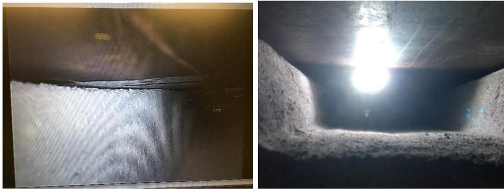
**Figure 63. Image capture of the inner concrete wall of the mock-up (left) and the mini inspection tool reaching the end of the refractory slot (right).**
