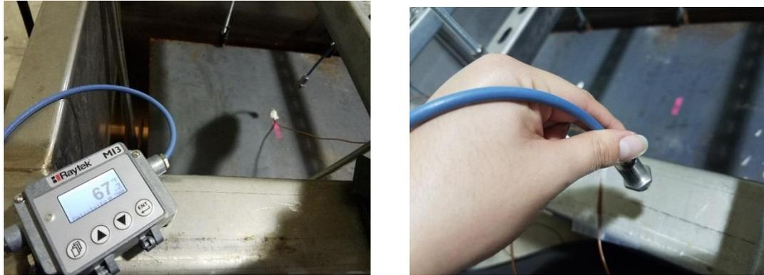
**Figure 85. Emissivity experiment with Raytek sensor a) carbon steel plate b) stainless steel tank wall.**
