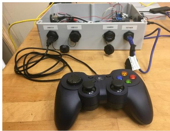
**Figure 48. Xbox controller attached to the controller box to provide the operator with the option of controlling both the mini inspection tool and the cable management system manually.**
