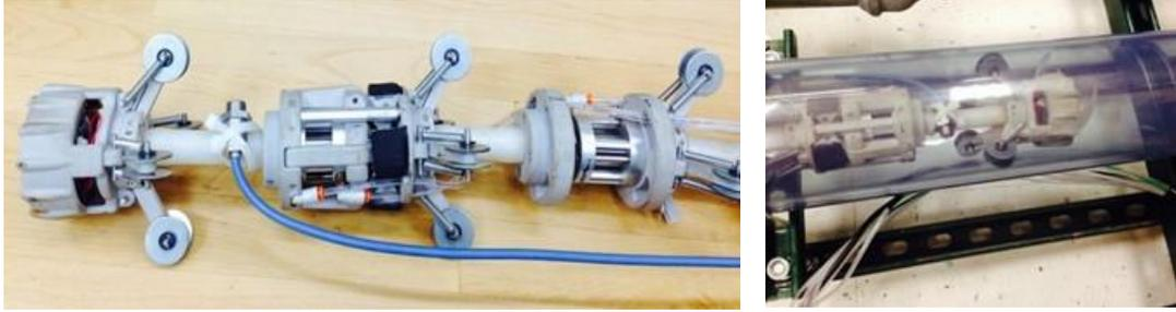
**Figure 88. a) IR sensor head on the pneumatic pipe crawler b) sensor head and crawler inside the clear pipe.**
