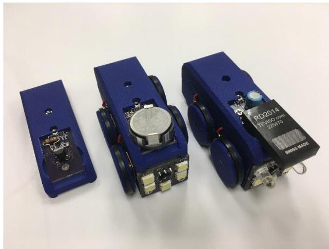
**Figure 46. Temperature sensor hood (left), inspection tool fitted with iButton humidity and temperature sensor (middle), and inspection tool fitted with RD2014 radiation sensor (right). The sensor hoods share common electrical and communication interfaces.**
