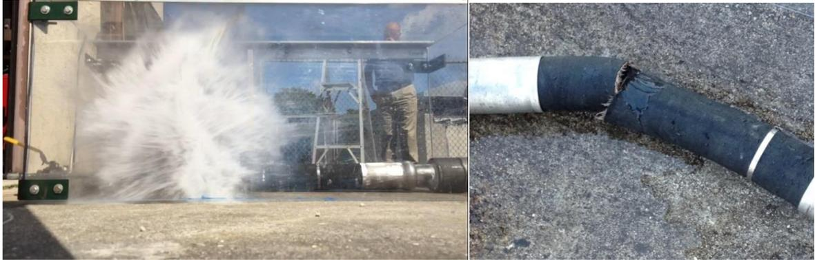
Figure 98. Ruptured hose section.
